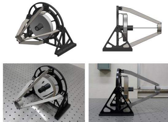
Figure 4. 3D model of SMT telescope (above) and Manufactured view (below)
