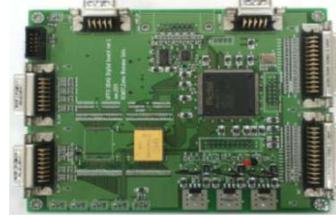
Figure 2: UFFO Data Acquisition (UDAQ) board
