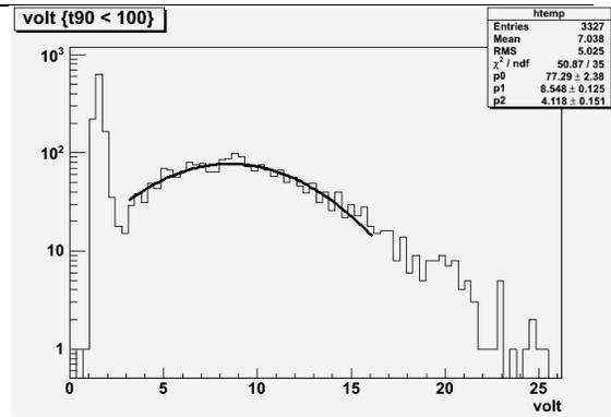
Figure 3: Amplitude distribution in mV. One photoelectron corresponds to 8mV amplitude.
