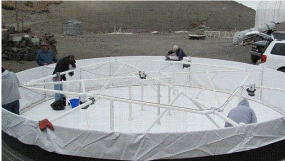
Figure 1: Photodetectors set up. PMTs are distributed at 2.4 m from the center of the tank, with a regular separation. One more is at the center of the detector.
