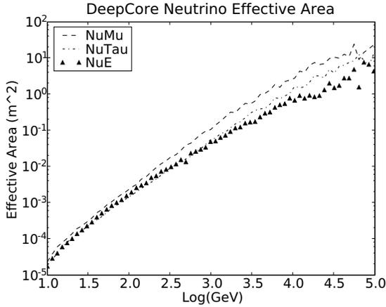
Figure 2: Effective area of the DeepCore detector given standard DeepCore SMT3 triggering for all flavor ( $\nu_e$ -triangle symbols,  $\nu_\mu$ -dashed line,  $\nu_\tau$ -dashdot line). The effective area has been averaged over the entire sky.
