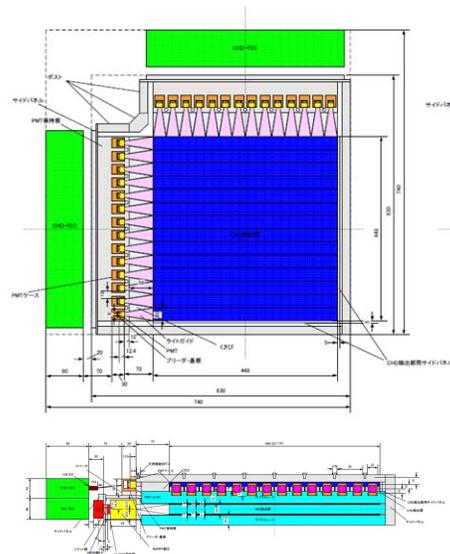
Figure 2: Structural design of CALET-CHD. The top (upper) and side (lower) views are shown. CHD is stacked up on the first layer of IMC.
