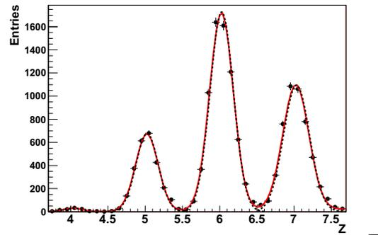
Figure 4: Nuclear charge spectrum obtained with a prototype scintillator paddle in GSI test. Peaks corresponding to  $Z = 4 - 7$  were fitted with Gaussian.
