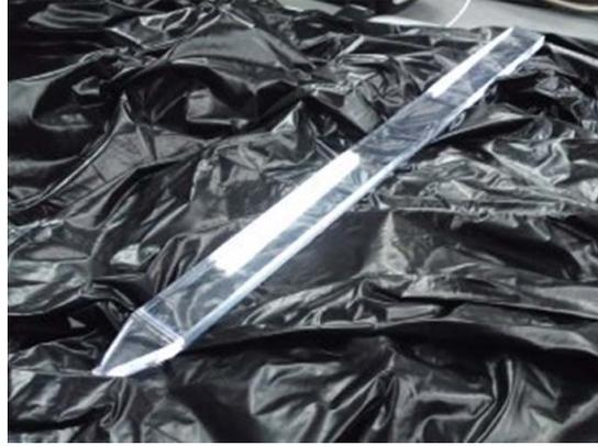
Figure 3: Picture of a prototype scintillator paddle of CALET-CHD. The paddle is composed of EJ204 scintillator and an acrylic light guide.
