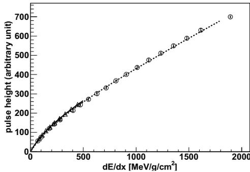
Figure 5: Correlation plots of  $dE/dx$  versus the pulse height of EJ204. Results from fragments generated from 500 MeV/nucleon Fe (circle) and 800 MeV/nucleon Si (triangle) in HIMAC test are shown. Fitting curves for Fe and Si data are shown by dashed and solid lines, respectively.
