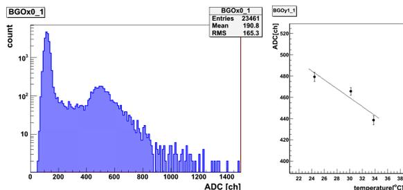
Figure 2: Distribution of ADC counts during muon-run (left), and the temperature dependence(right)
