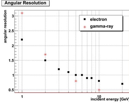
Figure 6: Expected angular resolution by simulation
