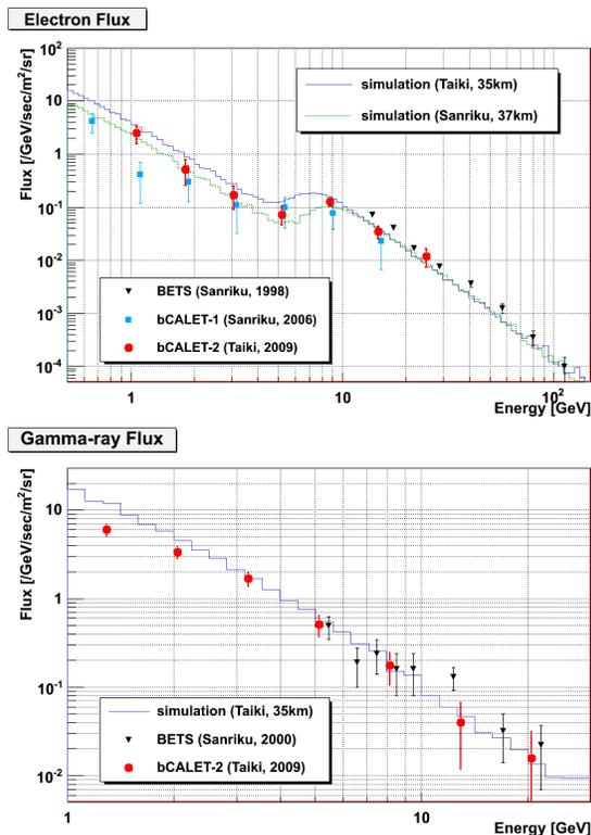
Figure 11: bCALET-2 results of electron and gamma-ray flux compared with previous experiments and simulation
