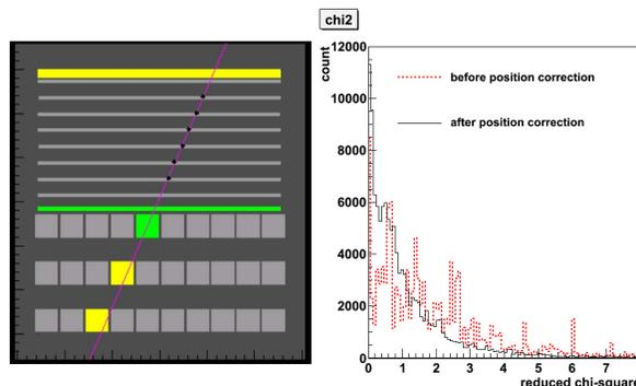
Figure 3: Example of muon track reconstruction(left), and distribution of chi-square values in muon track fitting before and after position correction(right)
