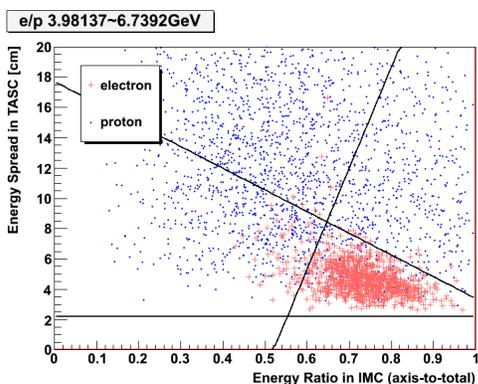
Figure 10: Correlation map of the lateral spread in TASC and the energy concentration in IMC (simulation)
