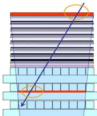
Figure 4: The events which pass through both the top of the detector and the third BGO layer are analyzed
