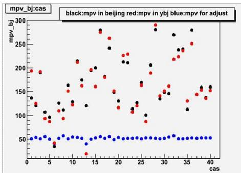
Figure 3. Mean amplitudes of all detector units in case of single particle measured in Beijing (black), at Yangbajing (red) and after high voltage adjustment (blue).
