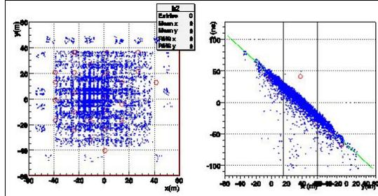
Figure 6. An example shower front observed by ARGO-YBJ (blue) and the KM2A engineering array (red). The green line in the right shows the shower plane reconstructed by the engineering array data.
