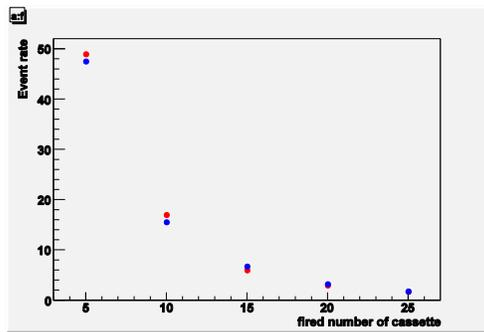
Figure 7. The measured trigger rates vs. event trigger threshold (blue) is consistent with that estimated by the ARGO-YBJ data (red).
