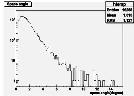
Figure 9. Distribution of space angles between the shower directions measured by the KM2A engineering array and the ARGO-YBJ experiment.
