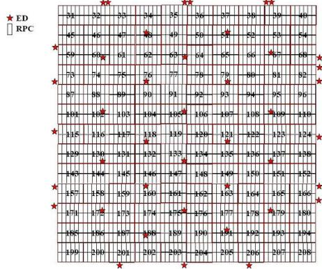
Figure 2. Sketch map of the KM2A engineering array in the ARGO-YBJ array. Each red star represents a detector unit.
