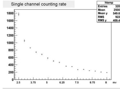
Figure 4. Single channel counting rate vs. threshold value.
