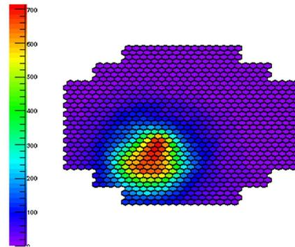
Figure 3: Simulated response of one H.E.S.S. camera triggered by a high energy proton shower. Each pixel represents a camera photo multiplier tube. The scale is the measured light intensity in units of photo electrons.
