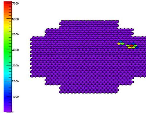
Figure 2: Simulated response of one H.E.S.S. camera triggered by a magnetic monopole event. Shown are two different clusters of pixel that are triggered by Cherenkov photons. Each pixel represents a camera photo multiplier tube. The scale is the measured light intensity in units of photo electrons.
