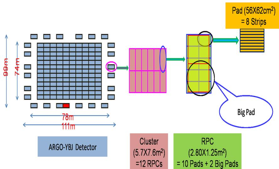
Figure 1: The ARGO-YBJ detector layout.
