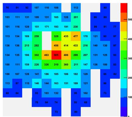
Figure 2: The particle density distribution of an EAS multicore event observed by the ARGO-YBJ detector. The sampling unit is the BigPad. For each BigPad the particle density is shown. The two BigPads with the maximum densities are indicated. Empty boxes correspond to poor functioning of the BigPads which are not used.
