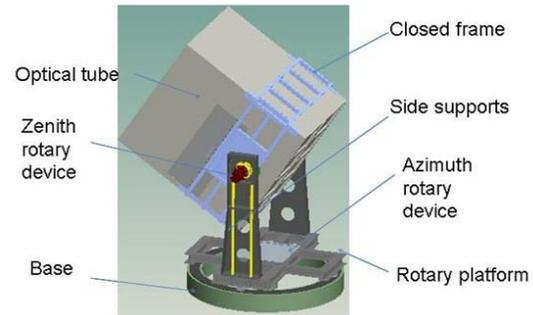
Figure 3: The mechanical structure of detector
