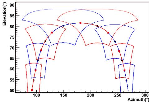
Figure 1: The trace of Crab Nebula in the local coordinates with the FOV of the telescope. The red and blue boxes indicate the FOV of the telescope in the local coordinates. The black dots show the center of the FOV of the telescope (the pointing of the telescope). The red dots indicate the pointing of the telescope is changed.
