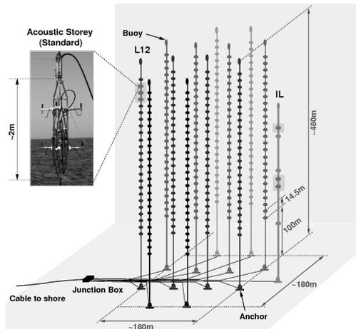
Figure 1: A sketch of the ANTARES detector. The six acoustic storeys are highlighted and a photograph of a storey in standard configuration is shown. L12 and IL denote the 12th detection line and the Instrumentation Line, respectively.
