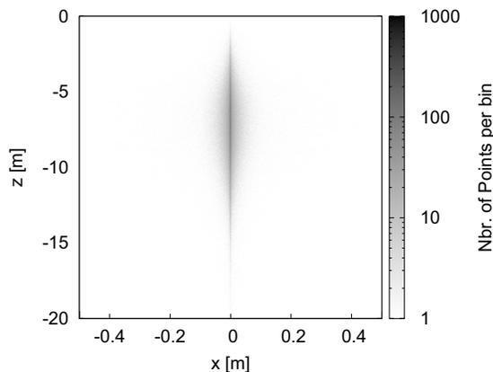
Figure 5: Density of the energy deposition of a  $10^{10}$  GeV hadronic shower resulting from a neutrino interaction, projected from a three-dimensional distribution upon the  $xz$ -plane. Bin sizes are 0.01 m in  $x$  and 0.1 m in  $z$ .
