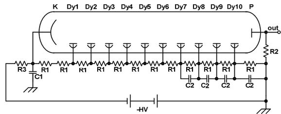
Figure 7. Schematic drawing of a voltage divider.
