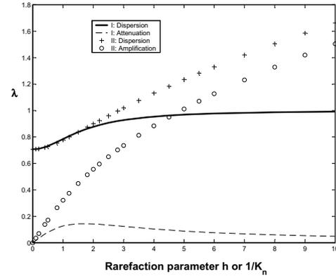
Figure 3: Dispersion relations of branches I and II over a range of  $h$  (rarefaction measure).  $\lambda_r$  : phase speed dispersion,  $\lambda_i$  : attenuation or amplification.  $\lambda = \lambda_r + i \lambda_i$ .  $\theta = 0$  here. Branch II (diffusion mode) shows anomalous amplification.
