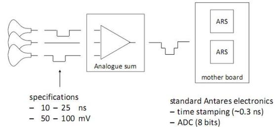
Figure 6. The principle of the analogue summing board.
