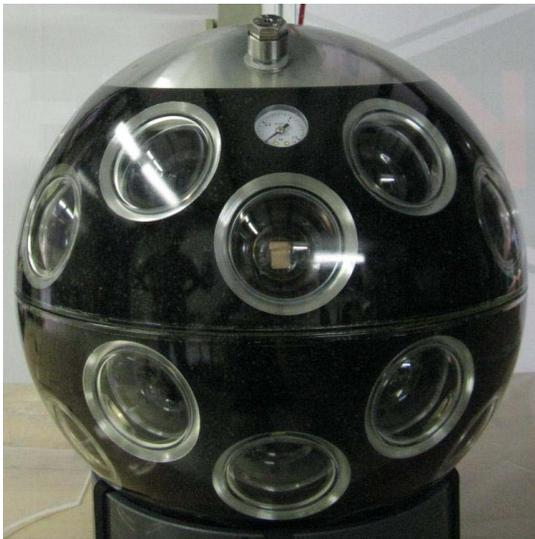
Figure 2. View of a KM3NeT prototype DOM.
