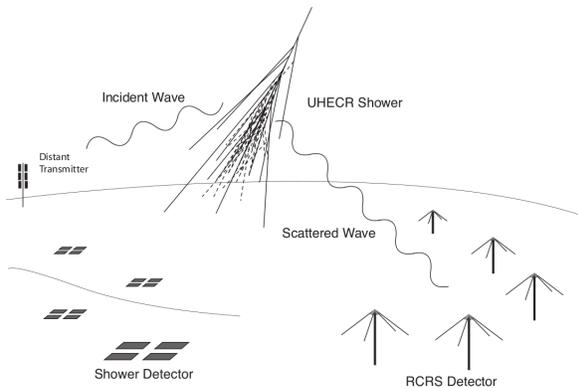
**Figure 1: The bistatic radar technique, as pioneered by the MARIACHI experiment. Conventional surface detectors are used to tag the presence of air showers while radar receiver stations detect the forward scattered echo.**
