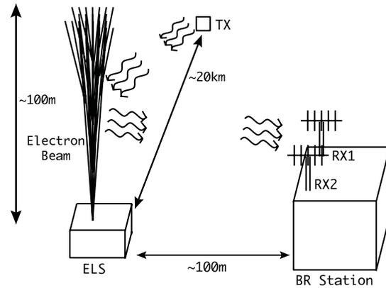
**Figure 6: Plan for radar studies in conjunction with the Telescope Array's Electron Light Source (ELS). Receiver antennas will be placed at right angles to a line joining the transmitter and 40 MeV ELS electron beam. Two antennas will be separated by one half-wavelength, to allow suppression of the direct illumination by the transmitter.**
