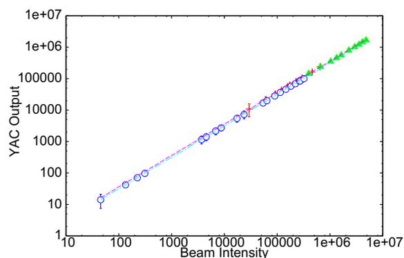
Figure 8: The saturation effect of the YAC. This figure shows that, within the experimental errors, there is a good linearity between the incident particle flux and YAC-ADC output below  $5 \times 10^6$  MIPs.
