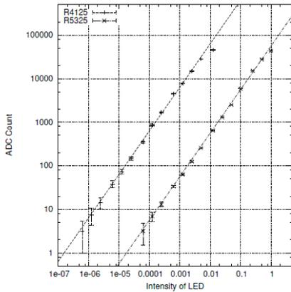
Figure 3: PMT R4125 and R5325 calibration by LED light source.
