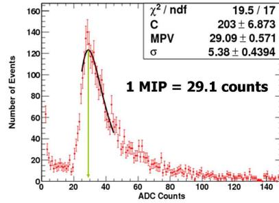
Figure 5: Charge distribution of single muons in a YAC detector. The peak is defined as one MIP. The resolution of ADC count is 0.25 pC/count.
