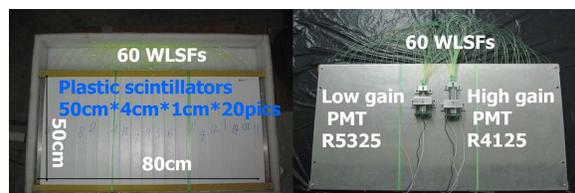
Figure 2: Each YAC's scintillation counter consists of 20 slabs of scintillator whose size is  $50 \text{ cm} \times 4 \text{ cm} \times 1 \text{ cm}$ , and light-isolated from each other using reflecting material. 20 WLSFs installed in the scintillators attached to the PMT R5325, the other 40 WLSFs attached to PMT R4125, that are responsible for the dynamic range of  $1-5000$  and  $10^3 - 10^6$ , respectively.
