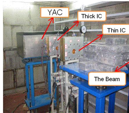
Figure 7: Electron beam calibration of YAC. From right to left, there are the beam, thick IC, thin IC and YAC scintillation counter.
