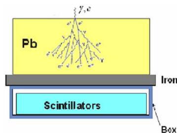
Figure 1: Each YAC detector unit consists of lead plates of 3.5 cm thick and a scintillation counter which detects the burst size induced by high energy electromagnetic component in the air-shower cores.
