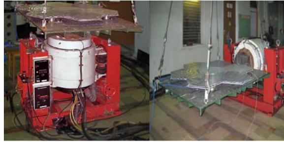
Fig.4. The technological Fresnel mirror at space qualification tests.
