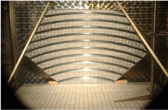
Fig.2. The mirror module test in thermo vacuum camera at temperature  $\pm 80^\circ\text{C}$  and pressure  $0.02 - 1.0\text{ atm}$ .
