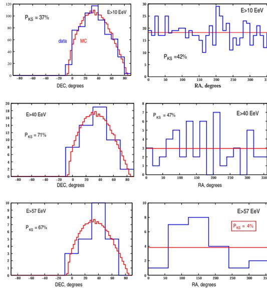
Figure 1: Comparison between the data (blue line) and the geometrical exposure simulations (red line) at energies 10 EeV, 40 EeV and 57 EeV (top, middle and bottom rows, respectively). Plots show the distribution of events in declination (right column) and right ascension (left column). The compatibility of the two distributions by the Kolmogorov-Smirnov test is given as  $P_{KS}$ .
