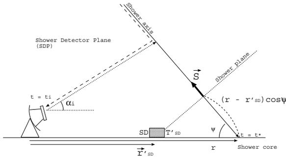
Figure 1: Shower detector plane and the time fit. In this analysis, we assume the shower front to be a flat plane.
