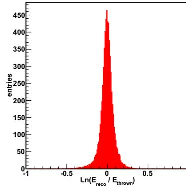
Figure 2: The energy resolution by the hybrid technique. The horizontal axis is natural logarithm of the reconstructed energy over true simulation energy. The vertical axis is the number of events. The standard deviation is 7%.
