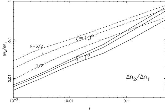
Figure 1: Ratio of the flux of the second to the first generation from flash ( $t = 0$ ) of a point source in a real atmosphere as function of  $\epsilon = ct/R - 1$ . Source is at zenith angle  $75^\circ$ . Lines (solid for  $\zeta = 1^\circ$ , dashed for  $10^\circ$ ) are for  $k = R/\lambda_{eff} = 0.5, 1.0, 1.5$  from bottom up.
