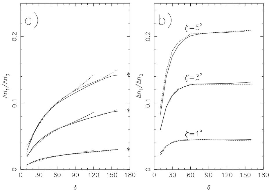
Figure 5: Ratio of the first generation to the direct light as function of angle  $\delta$  between shower and line of sight. Solid lines - exact numerical calculations, dotted lines and stars in a) - analytical (approximate) calculations, dashed lines - our parametrization of the numerical curves (eq. 4-7). All curves are for  $k_Q = R/\lambda_Q = 1$ .
