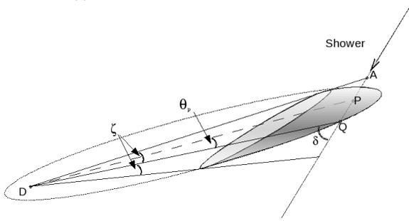
Figure 2: Fluorescence light produced at point  $P$  and scattered on the shaded part of the ellipsoid arrives at the detector  $D$  simultaneously with the direct light prod. at  $Q$ .
