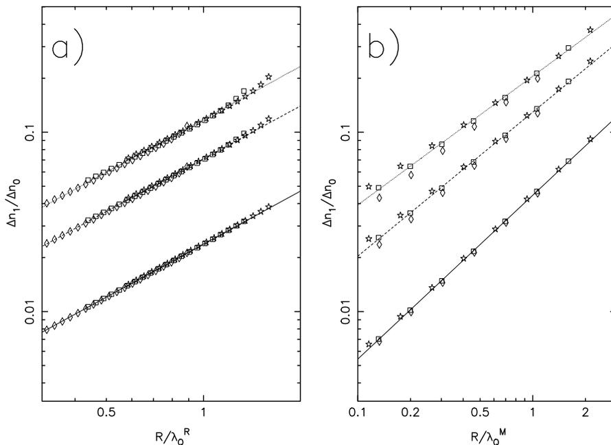
Figure 4: Ratio of the first generation to the direct light as a function of distance  $R$  to point  $Q$  on the shower in units of the scattering length  $\lambda_Q$  at that point. a) Rayleigh, b) Mie scattering. Curves correspond to  $\zeta = 1^\circ, 3^\circ, 5^\circ$  and  $\delta = \pi/2$ . Various point shapes refer to different distances  $R=12, 24, 32$  km. Lines are power law fits.
