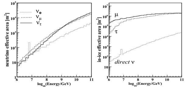
Figure 4: The left panel shows  $4\pi$  solid angle averaged neutrino effective areas for each neutrino flavor. The dashed line corresponds to  $\nu_e + \bar{\nu}_e$ . The solid line is  $\nu_\mu + \bar{\nu}_\mu$ , and the dotted line is  $\nu_\tau + \bar{\nu}_\tau$ . All assume equal flux of neutrinos and anti-neutrinos. The right panel shows the effective detection area near the detector for secondary muons, taus and primary all flavor neutrinos.
