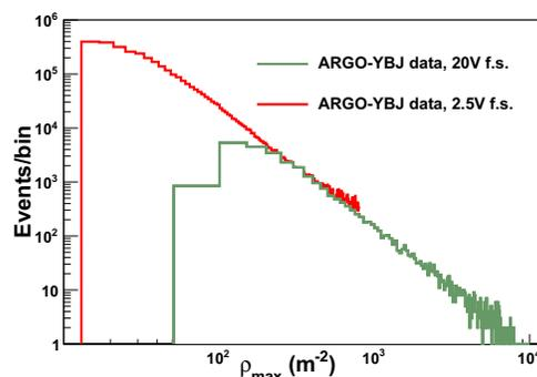
Figure 2: Histogram of the maximum particle density ( $\rho_{max}$ ) as measured by ARGO-YBJ at two f.s. (2,5 V (red) and 20 V (green)) of the analog readout.
