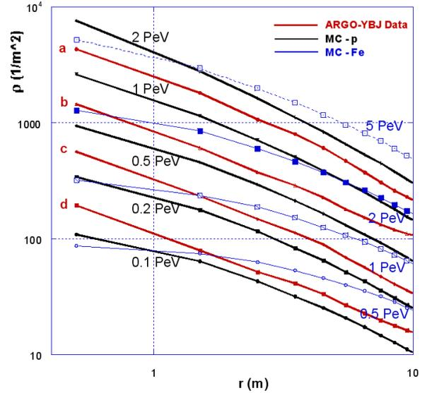
Figure 4: Lateral distribution for data (red lines) for 20 V and 2.5 V f.s. data (see text); the black lines are MC predictions for protons at 100 TeV (the lowest), 200 TeV, 500 TeV, 1 PeV, and 2 PeV (the highest); the blue lines are MC predictions for irons at 500 TeV (the lowest), 1 PeV, 2 PeV and 5 PeV (the highest).
