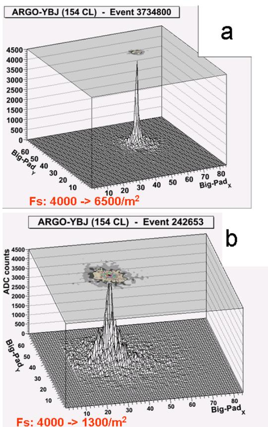
Figure 1: Showers as recorded by ARGO-YBJ through the analog readout system, respectively at 20 V f.s. (a) and 2.5 V (b).
