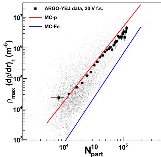
Figure 6:  $\rho_{max} \times (\partial\rho/\partial r)_1$  vs  $N_{part}^{10}$  for data (see text for details) along with expectations both for proton (red line) and iron (blue line) induced showers. The black dots are from profile in  $8 \cdot 10^3 \leq N_{part}^{10} \leq 1.1 \cdot 10^5$
