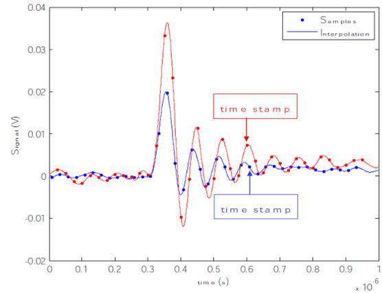
Figure 4: Typical waveforms from a charge amplifier with 50ns peaking time, measured with a digital oscilloscope at a sampling rate of 40MS/s and then interpolated. Note the asynchronous samples. This particular amplifier suffered from some ringing, but this is irrelevant to the measurement.
