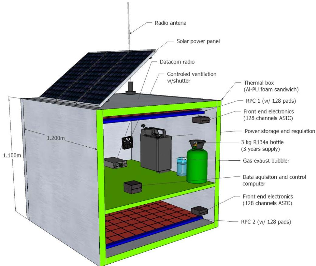
Figure 1: Conceptual representation of a tracking standalone RPC station. It is clear that if standalone operation is not required the communications and the gas and power supplies may be advantageously housed at a nearby station.
