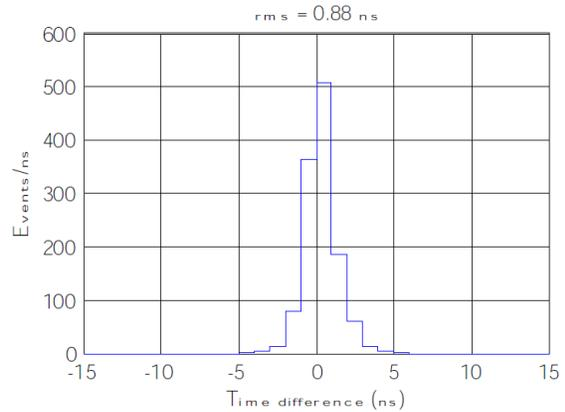
Figure 5: Distribution of the measured time difference, with an rms of 0.88ns.
