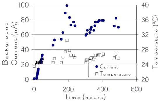
Figure 3: Evolution of the dark current as a function of time after the gas flow was reduced to 1 kg/year, at the nominal working voltage of 5600 V.
