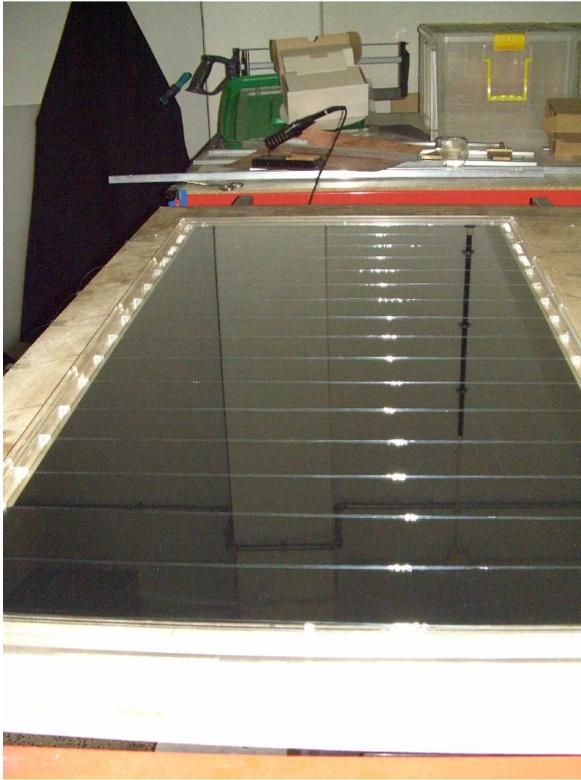
Figure 2: Double-gap RPC module with  $0.5 \times 1\text{m}^2$ . The RPC is completely contained inside an impermeable high-voltage and gas enclosure.
