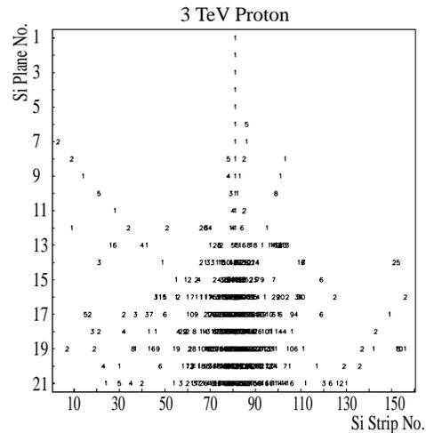
**Fig.2** Typical 3 TeV proton as seen by the ELO calorimeter.
