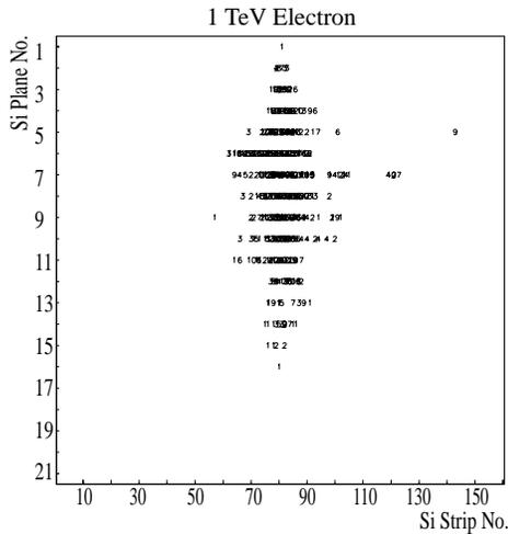
**Fig.1** 1 TeV electron as seen by the ELO calorimeter. The numbers within the graph represent the number of mips (minimum ionizing particles) recorded by each strip.
